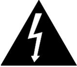
The arrowhead symbol on a lightning flash inside a triangle is intended to alert the user to the presence of un-insulated "dangerous voltage" within the enclosed product which may be of sufficient magnitude to constitute a risk of electric shock to persons.
